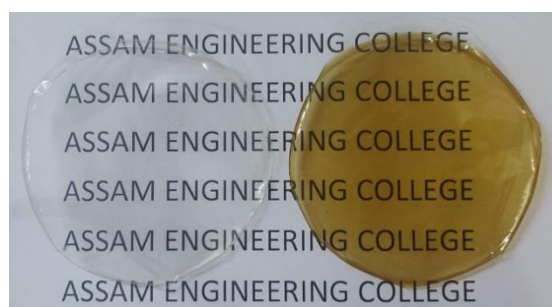
Figure: Seaweed biopolymer film (a) without carbon dot (b) with carbon dot
