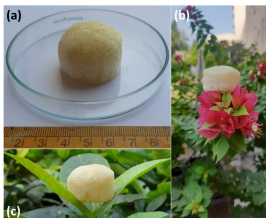
Fig. Digital photographs of water-soluble and biodegradable foams prepared using gelatin.
